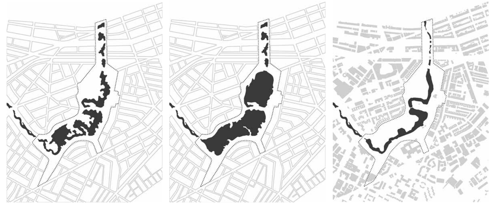
ABOVE Student diagrams depict water surface at low tide (left) and high tide (center), indicating the storage capacity of the Back Bay Fens in the original design, and water surface in 2017 (right).
